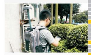
In addition, S650 and S660 enable to use a variety of PDA mobile terminal with all kinds of operating system, such as *Andriod, IOS, WIN7/WIN8*, even more Windows mobile. Cellphone, tablet are the best choice data collectors to work with S650 and S660 to connect to network, improve flexibility for fieldwork. In combination with communication module of mobiles, S650 and S660 get a faster way to obtain correction from CORS network.
