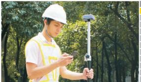
South S650/660 gnss receiver, adopts market-proven Pacific Crest Maxwell 6 technology (BD910/BD930 OEM board), 220 channels and unmatched gnss multiconstellation tracking performance, makes effective use of GPS and GLONASS signal for outstanding satellite coverage and high precise positioning.
